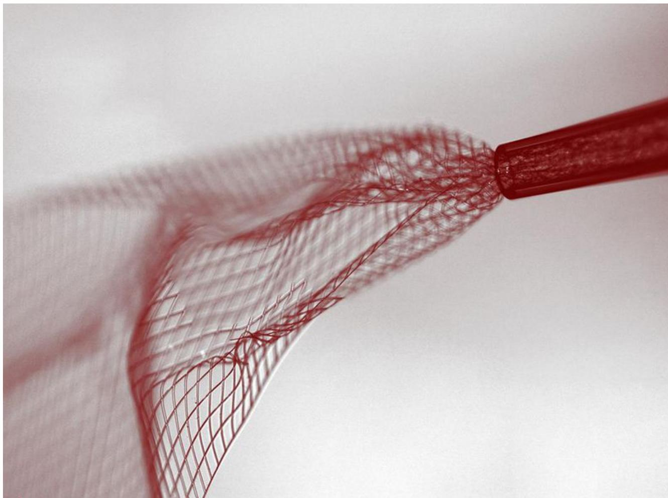
The rolled electronic mesh is injected through a glass needle into a water-based solution. (Lieber Research Group, Harvard University)
